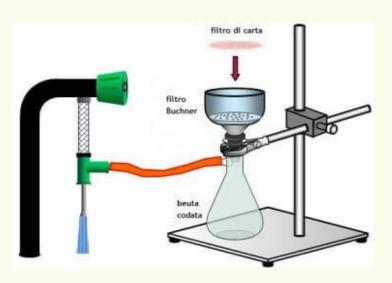
filter, start the vacuum (open the tap!) and go. When the filtration slows down, the filter with the accumulated mass is carefully removed and set in a beaker and a new filter is placed in the funnel. At the end of filtration — which is neither painless nor very fast; remember to wear gloves and face protection — collect as much of the precipitate as possible from the filters, while discarding the liquid in the flask, consisting of water and NH<sub>3</sub>. Add more water, dilute, etc.
